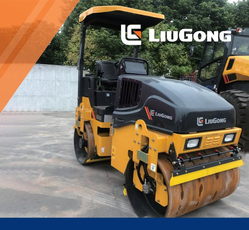
EnginePerkins 403D-15TRated Power27.3 kW (36 hp / 37 ps) @ 2,600 rpmNominal Amplitude Range0.45 mmVibration Frequency Range60 HzCentrifugal Force Range33.5 kNWorking Width1,200 mmOperating Weight3,360 kg
