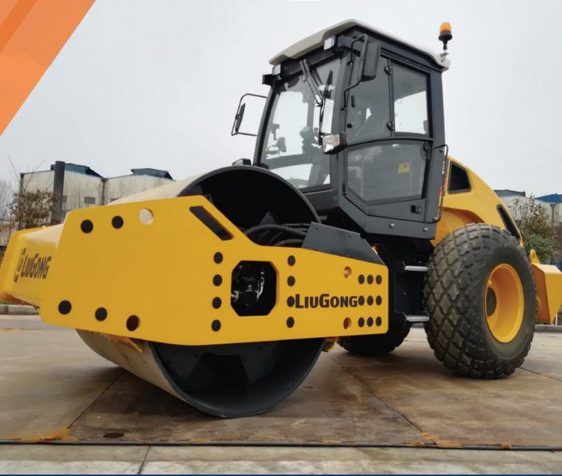
Engine Rated Power Nominal Amplitude Range Vibration Frequency Range Centrifugal Force Range Working Width Operating Mass CUMMINS QSB4.5 119 KW (160 HP) @ 2,200 RPM 2.0 / 1.2 MM 30 / 33 Hz 300 / 220 kN 2,130 mm 13,200 kg
