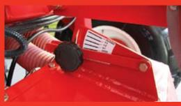
When double shooting, a fully adjustable plenum lets you divert more air to the meter with heavier products and higher rates of application, and less with lighter or more fragile products.
