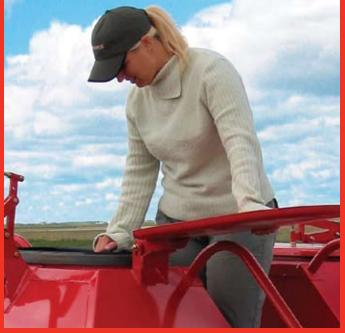
The walk-through tank design creates a firm standing platform with fill lids at waist level.
