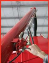
The 7000 Series auger is double-hinged for exceptional balance, allowing one person to easily load and unload. The 7180 model is equipped with a 7" auger. The 7240 and 7300 models come with 8" auger.
