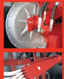
On the MORRIS system, product does not have to be lifted and experiences no 90-degree bends or sharp turns, so only one fan is required to move product from the meter bodies to the ground. An industrial piston-type hydraulic motor powers a 13" (33 cm) diameter forward curved fan that is 98% efficient. Use of larger hydraulic lines decrease flow restrictions for less heat buildup under higher fan speeds.
