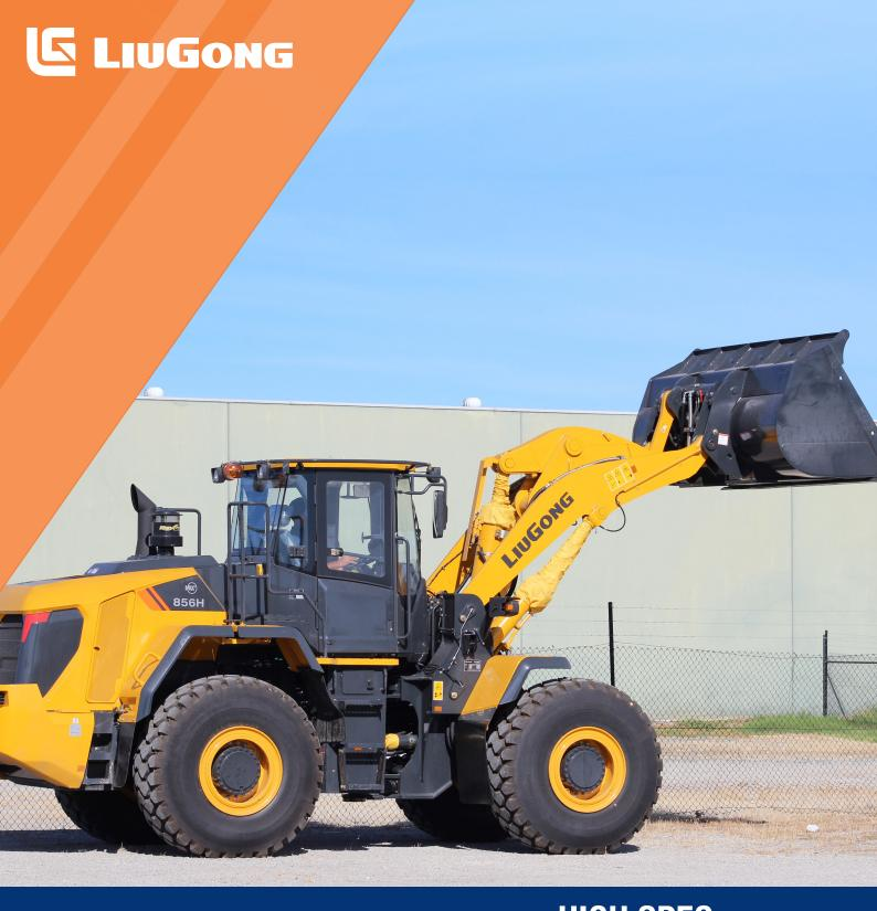
EngineCummins QSL9.3Rated Power162 kW (217 hp / 220 ps) @ 2,200 rpmNet Power162 kW (217 hp / 220 ps) @ 2,200 rpmOperating Mass19,500 kgStandard Bucket Size3.5 M³Standard Breakout Force161 kNStandard Dump Clearance2,978 mm
