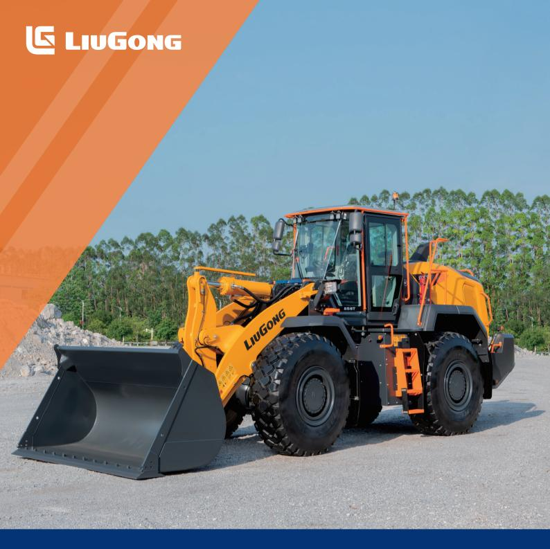
EngineCummins L9Rated Power170 kW (228 hp / 231 ps) @ 2,000 rpmOperating Weight19,500 kgStandard Bucket Size3.5 m³Standard Breakout Force152 kNStandard Dump Clearance2,697 mm
