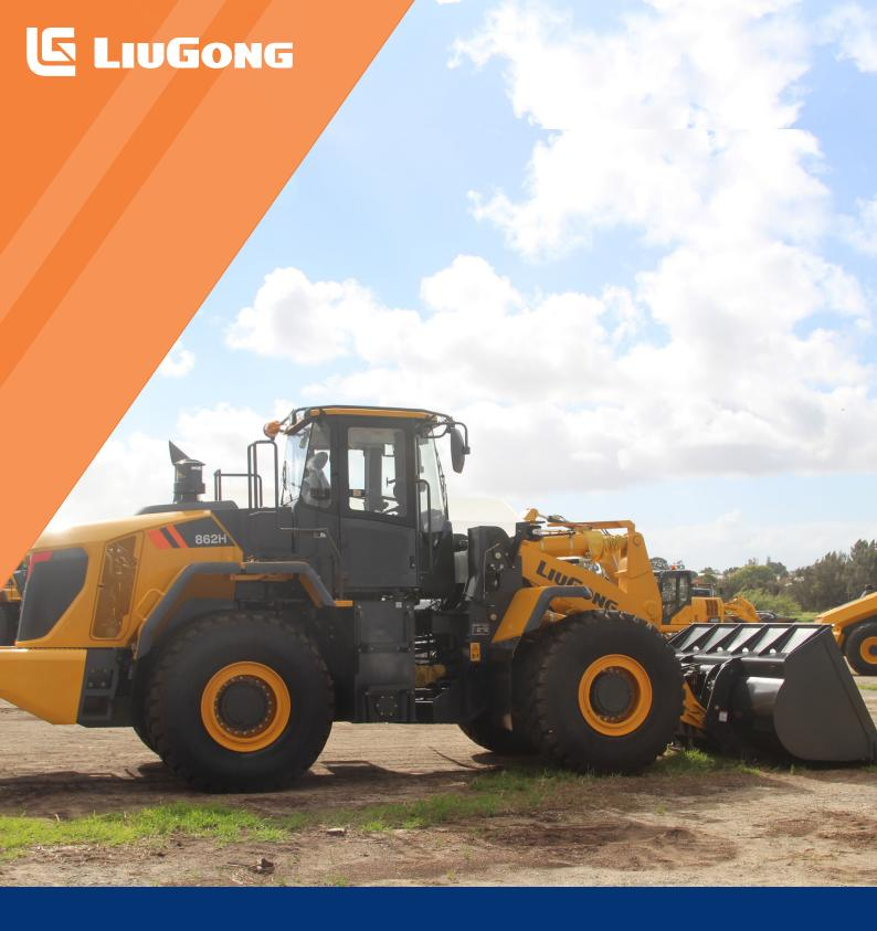
EngineCummins QSL9.3Rated Power180 kW (241 hp / 220 ps) @ 2,200 rpmNet Power180 kW (241 hp / 220 ps) @ 2,200 rpmOperating Mass21,420 kgStandard Bucket Size4 M³Standard Breakout Force175 kNStandard Dump Clearance3,225 mm
