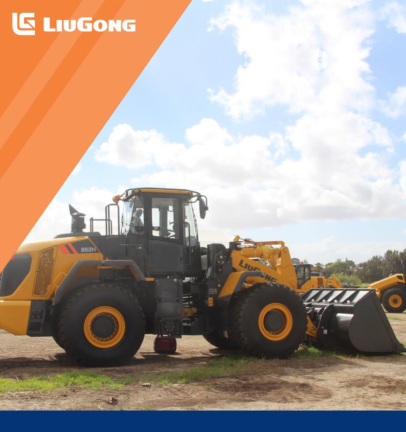
EngineCummins QSL9.3Rated Power180 kW (241 hp / 220 ps) @ 2,200 rpmNet Power180 kW (241 hp / 220 ps) @ 2,200 rpmOperating Mass21,500 kgStandard Bucket Size4 M³Standard Breakout Force175 kNStandard Dump Clearance3,225 mm
