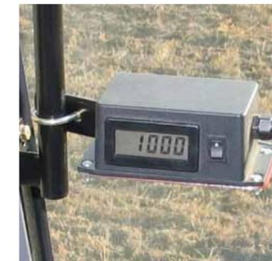
Once set, pressure can be adjusted from the tractor cab on a convenient digital display.
