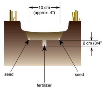
The **paired row double shoot opener** places 2 distinct rows of seed 10 cm (4") apart. Seed is first placed in two distinct rows 5 cm (2") to each side of the knife followed by a fertilizer band that is placed directly behind the knife and 2 cm (3/4") below the seedbed. This patented design results in outstanding fertilizer - seed separation and improved seed bed consistency through minimizing soil fracturing.
