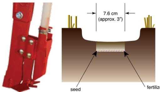
The **spread tip single shoot opener** places a 7.6 cm (3") wide ribbon of seed in each seed row. This opener cuts a smooth level seedbed resulting in very consistent seed placement and has been designed to minimize soil disturbance. The spread tip opener, with its high seed bed utilization is an excellent choice for farmers who apply low to moderate fertilizer rates with the seed.
