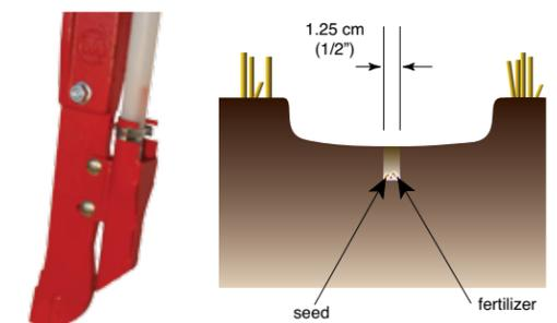
The **narrow knife single shoot opener** is a single shoot opener that places a narrow 1.25 cm (1/2") ribbon of seed in each seed row. This opener cuts a smooth narrow channel for seed to be placed, and has the lowest soil disturbance of the openers available. This opener has proven to be a popular choice with growers with sticky, high clay content soils.
