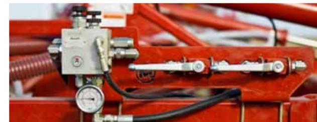
A hydraulic valve manifold providing all operator adjustments is conveniently located on the front bar of the drill.
