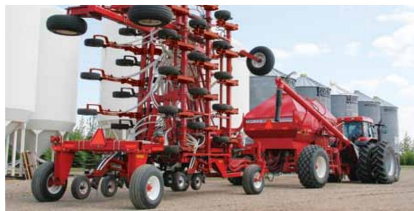
Narrow transport models in 25 feet and 31 feet widths. This is an ideal option for front wheel assist tractors in the 200 horsepower range.
