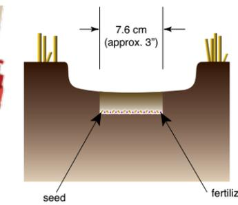
The **spread tip single shoot opener** places a 7.6 cm (3") wide ribbon of seed in each seed row. This opener cuts a smooth level seedbed resulting in very consistent seed placement and has been designed to minimize soil disturbance. The spread tip opener, with its high seed bed utilization is an excellent choice for farmers who apply low to moderate fertilizer rates with the seed.
