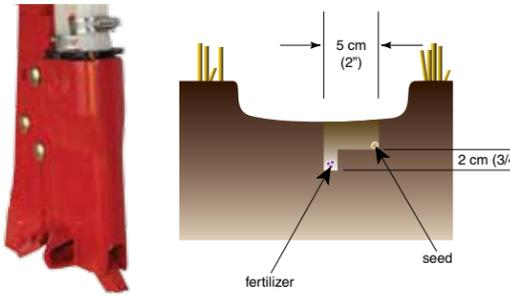
The **side band double shoot opener** first places a distinct seed row 5 cm (2") to the side of the knife followed by a fertilizer band which is placed directly behind the knife and 2 cm (3/4") below the seedbed. This patented design results in outstanding fertilizer - seed separation and improved seed bed consistency by minimizing soil fracturing.
