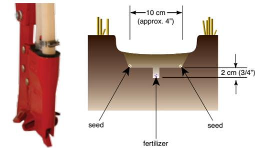
The **paired row double shoot opener** places 2 distinct rows of seed 10 cm (4") apart. Seed is first placed in two distinct rows 5 cm (2") to each side of the knife followed by a fertilizer band that is placed directly behind the knife and 2 cm (3/4") below the seedbed. This patented design results in outstanding fertilizer - seed separation and improved seed bed consistency through minimizing soil fracturing.
