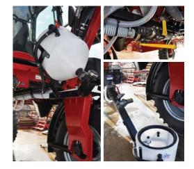
Mounted on a dropdown arm attached at the front of the machine and can be lowered and raised with an electric winch.
