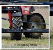
Major components carefully placed, so weight distribution is near 50-50 balance during spraying.
