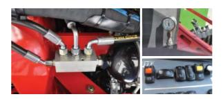
pressure on the implement's gauge wheels is automatically maintained through undulating terrain. This is operated in-cab and is activated or deactivated by the main lift switch on the joystick. This option acts as a "return to cut" function when swathing.
