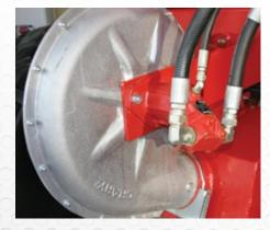
**High Flow Fan** The high-flow fan gives added product-carrying capacity. The fan's piston hydraulic motor is 98% efficient and rated for 10,000 hours of service.
