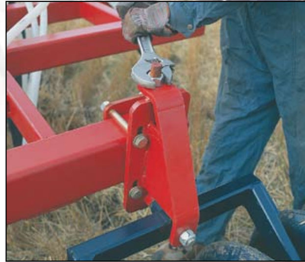
"Quick Adjust" packer brackets make levelling a quick and simple task.
