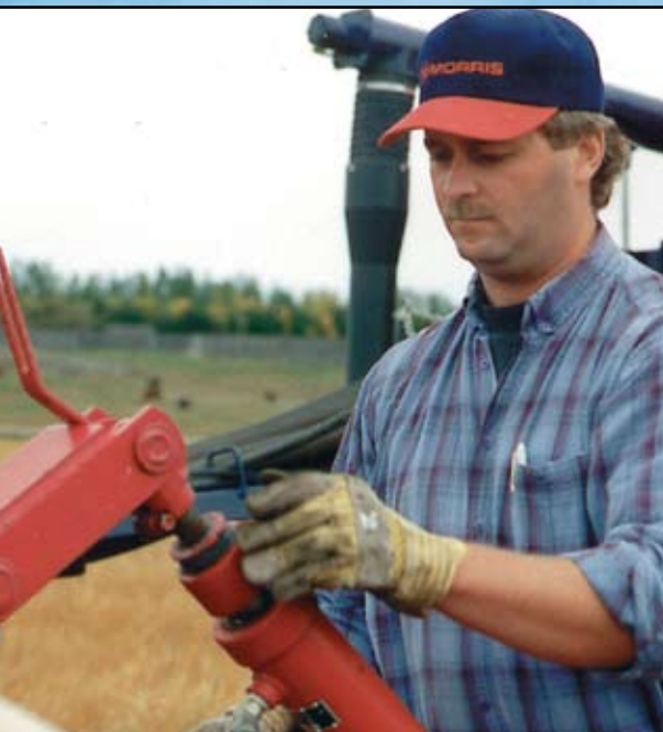
Depth stop collars ensure precise depth setting across the entire machine.
