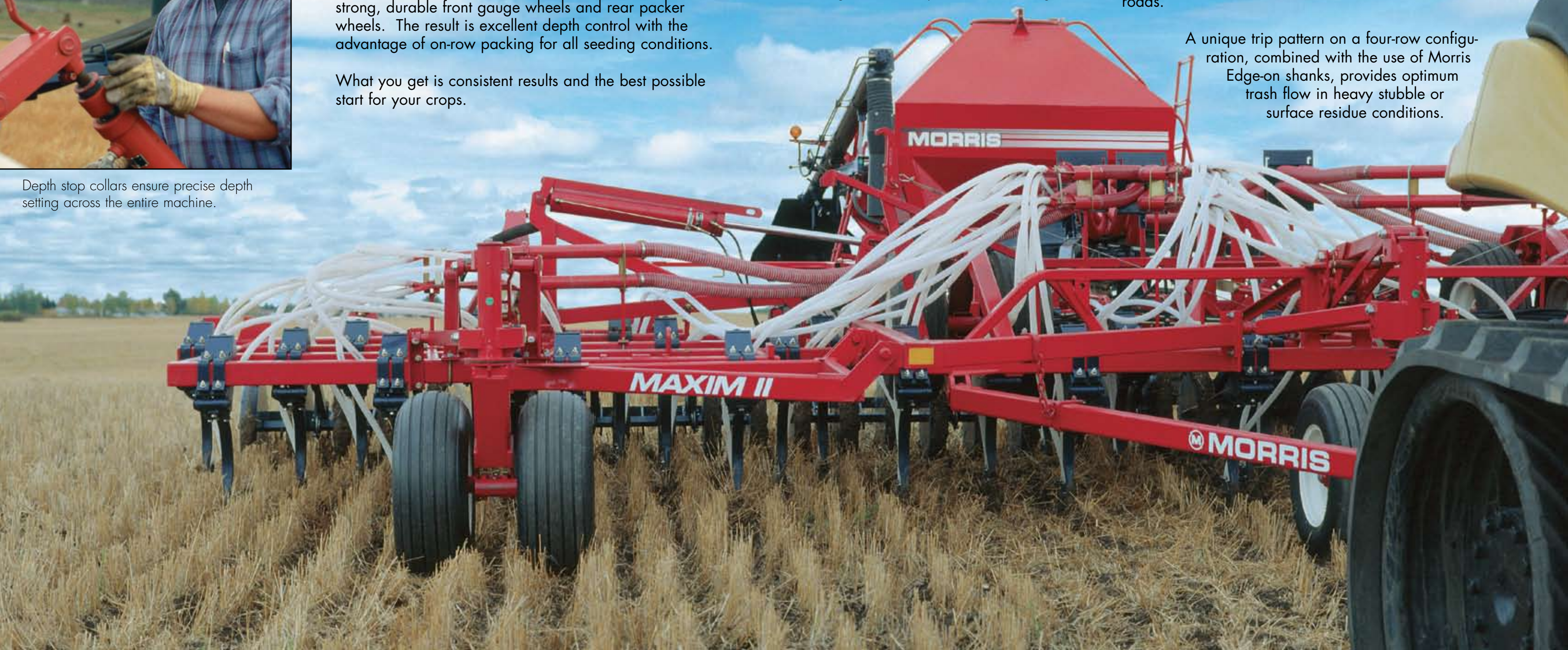
The Maxim II's clean, unobstructed under carriage allows heavy trash to flow through.
