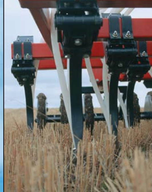
The Maxim II's clean, unobstructed under carriage allows heavy trash to flow through.
