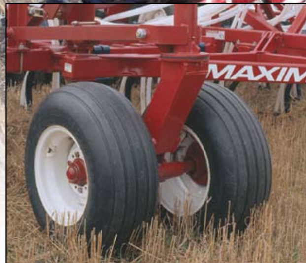
Offset dual gauge wheels walk right over clumps and rocks, reducing frame bounce for consistent seed depth.
