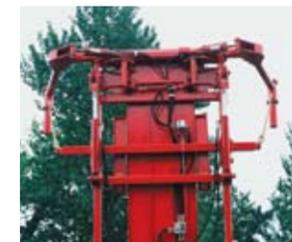
ProAG Bale Scoops feature a custom sequence valve and a 4-way valve to control the alignment arms, grab hooks and loader.
