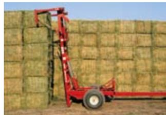
Fork lift teeth are sturdy enough to withstand impact and weight of a full stack of bales.
