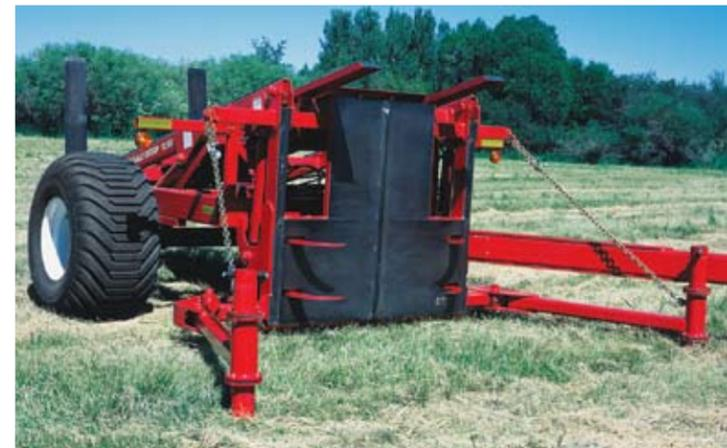
The Auto Align® system allows the operator to pick up bales in the same direction as the field was baled (12SR model shown).
