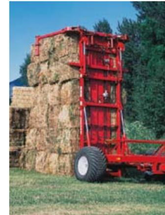
Once the bed is vertical, the alignment arms are opened, and the 12SR is driven forward to remove the teeth from under the stack.
