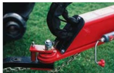
4x4 baler ball style hitch. Hydraulic hoses are sheathed and labeled for easy hook-up. Safety chain is included.
