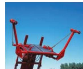
Grab hooks hold the first bale in place. Unique floating pipes on the alignment arms hold the second bale, to create the forward stair-step.
