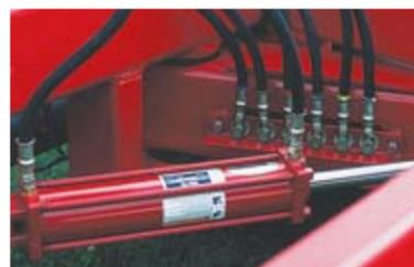
The hydraulic manifold (12SR shown) is located for easy access and servicing.
