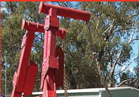
Optional Short Bale Bracket attachments can be mounted on the alignment arms to pick up shorter wet silage bales.
