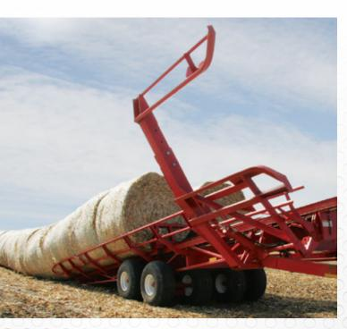
When unloading, the push bar travels all the way to the back, maintaining tight stacks. The adjustable bale divider has twelve positions to provide the operator the flexibility to set the bale spacing when unloading in the yard, providing the air circulation needed between the rows.
