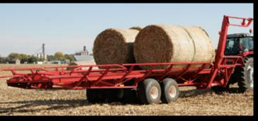
Only two hydraulic outlets are needed for full operation of the Bale Hiker.
