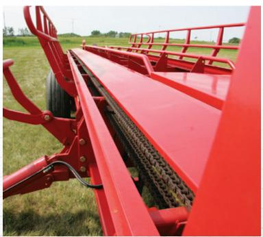
The smooth bed design protects net-wrap from tears, making it gentler than any other round bale carrier. Chains are completely covered and protected from dirt and debris that falls from the bales.
