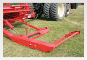
The robust heavy-duty bale fork adjusts to lift bales between 4 and 6 feet in diameter. Bale turners on the inside and outside of the fork allow bales to be picked in any direction. Right side picking reduces stress on the operator and eliminates weaving through the field.
