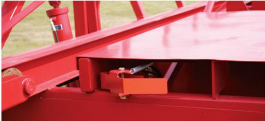
The full load indicator on the 2200 Bale Hiker signals the operator when the Bale Hiker has reached its maximum load capacity.
