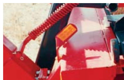
The full load indicator on the 1400 signals the operator when the Hay Hiker has reached its maximum load capacity.
