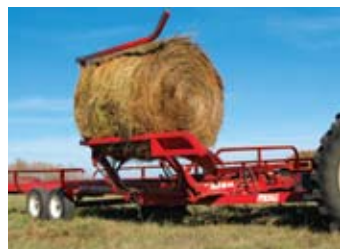
A selector valve provides a fail safe mechanism to prevent bales from being loaded in front of the push bar.
