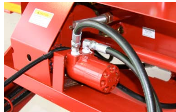
High capacity orbit motor is ideal for today's high performance tractor hydraulic systems. It ensures smooth operation with the most demanding loads.
