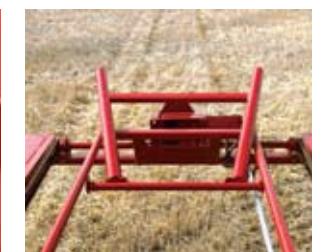
Bale dividers gently separate the bales as they are unloaded, creating air circulation between the two rows to prevent spoilage.
