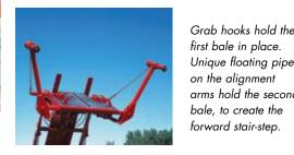
first bale in place. Unique floating pipes on the alignment arms hold the second bale, to create the forward stair-step.
