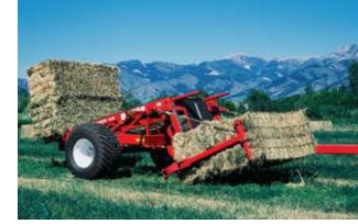
Automatic grab hooks hold the first bale in position, without dragging the bale, allowing the alignment arms to reopen to engage the second bale. The loader automatically rotates up as the two bales are
