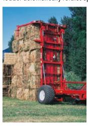
Once the bed is vertical, the alignment arms are opened, and the 12SR is driven forward to remove the teeth from under the stack
