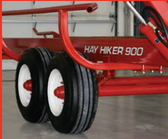
The 900 features heavy-duty axles, tires and 8-bolt hubs for exceptional load capacity.
