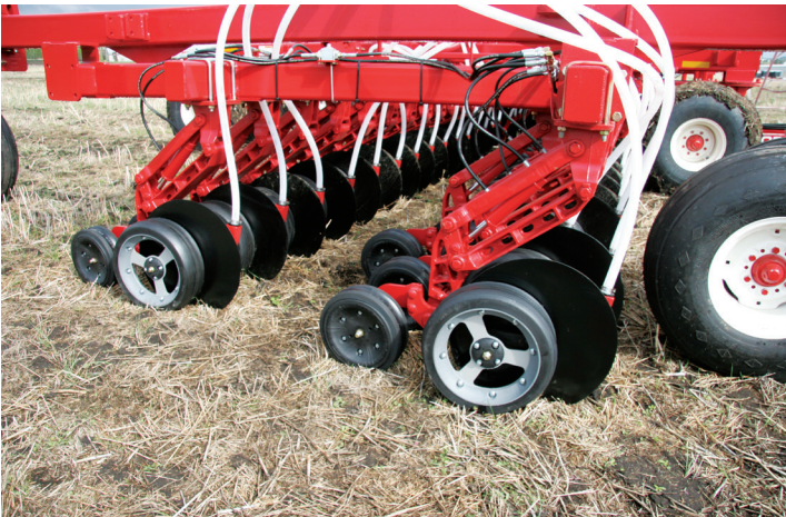
Walking beam design for better penetration ability at higher speeds
