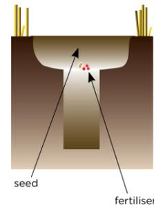
The **NARROW KNIFE SINGLE-SHOOT OPENER** is a single-shoot opener that places a narrow 125 mm (5") ribbon of seed in each seed row. This opener cuts a smooth narrow channel for seed to be placed, and has the lowest soil disturbance of the openers available.
