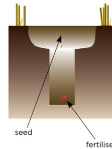
The **IN-LINE DUAL SHOOT OPENER** places fertiliser below the seed and leaves a narrow trench to maximise water harvesting. This option also has the greatest potential to utilise sub soil moisture through capillary action.
