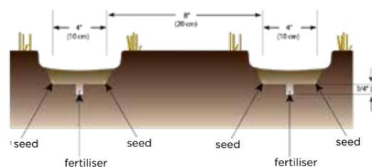
The **PATENTED PAIRED ROW DOUBLE-SHOOT OPENER** places two distinct rows of seeds 100 mm (4") apart with fertiliser placed centrally and 20 mm (3/4") below the seed rows.
