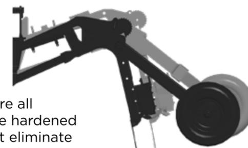
The linkage pivots are all 1" chrome pins inside hardened plastic bushings that eliminate steel on steel wear and negate the need for greasing.
