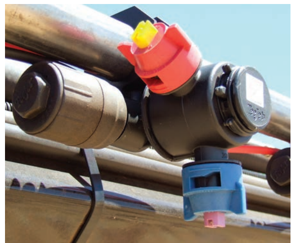
TeeJet Air-Chemsaver pneumatic shut off valves for rapid switching between SSC stages.
